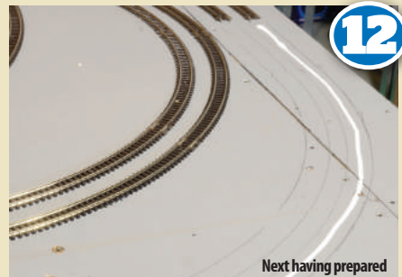
12 Next having prepared holes for point motors, the track was lifted and a bead of PVA glue run round the centre of the previously drawn pencil marks.
