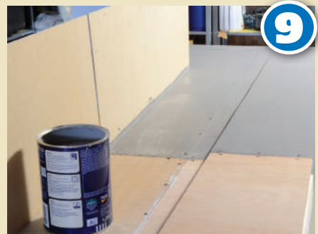
9 To improve the appearance of the fiddle yard all of the original track was lifted so that the baseboard surface could be painted grey. This also sealed the baseboard surface.
