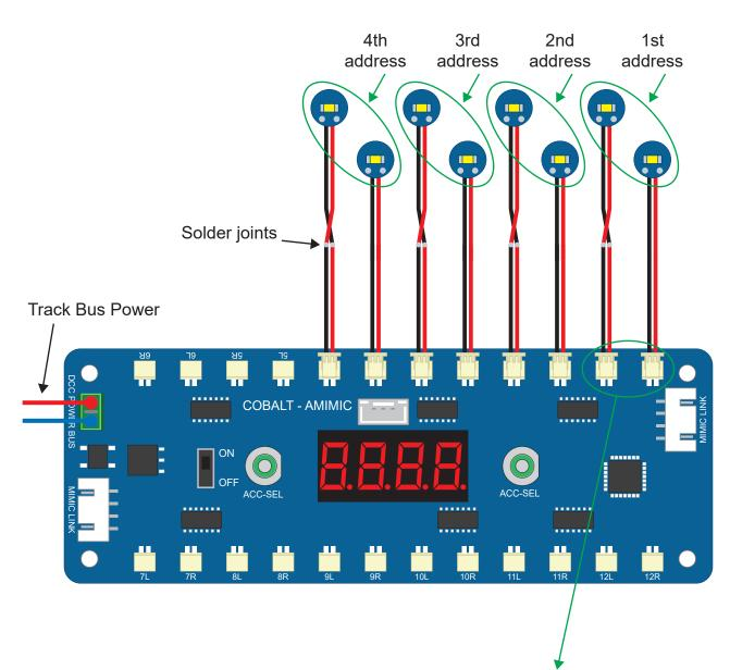
If the LEDs are on when they should be off, swap the two connections in the L and R sockets
