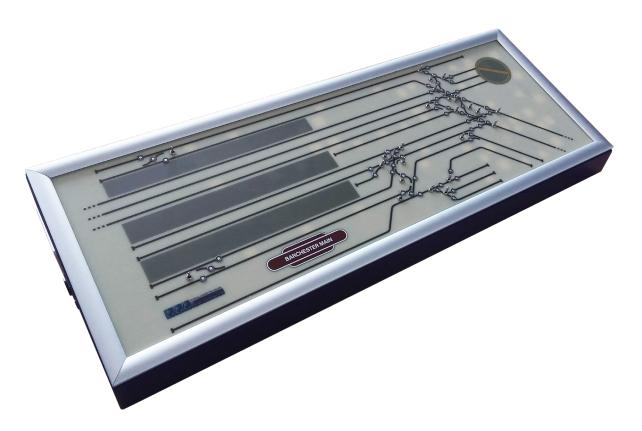
This control panel included a Super Panel, multiple Alpha Mimics, box size 4 and controlling 28 DCC accessory address.
