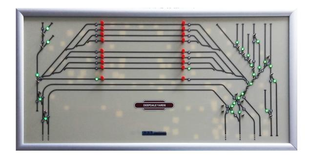
This control panel included a Super Panel, multiple Alpha Mimics, box size 5 and controlling 26 DCC accessory address. It also included route setting for the storage area via the Super Panel programming.
