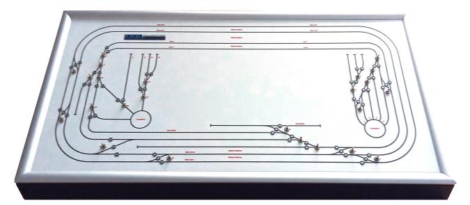
This control panel included multiple Alpha Encoder Units, Alpha Mimics, box size 5 and controlling 28 DCC accessory address.
