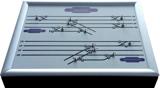
This control panel included an Alpha Encoder Unit, an Alpha Mimic, box size 3 and controlling 12 DCC accessory address.
